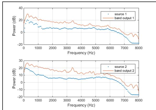
Fig. 3 The spectra of the original sources 1 and 2, and the separated signals at bands  $y_1$  &  $y_2$ .
