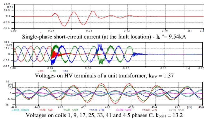
Fig. 2. Switching off a single-phase short-circuit at a distance of 0.25 of the line length from the unit transformer
