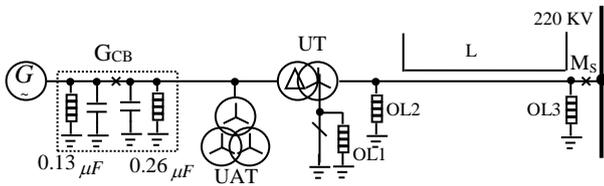
Fig. 1. Diagram of the modeled path of power evacuation from the power plant (G - generator 282 MVA, 15.75 kV; UT - unit transformer 270 MVA, 250 kV / 15.75 kV; UAT - unit auxiliary transformer 32 MVA, 15.75 kV / 6 kV / 6 kV; L - 220 kV two-circuit line, line length  $l_L = 22$  km; GCB - generator circuit breaker including capacitors and overvoltage limiters; M<sub>5</sub> - mains switch; OL1, OL2, OL3 - overvoltage limiters)
